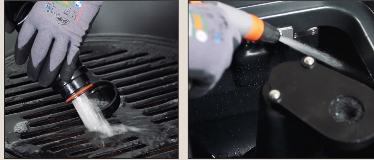
Empty and clean the recovery tank and floating system
