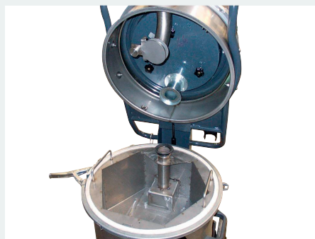
Tilting head for an easy removal of the basket and the bin
