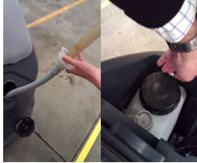
2. Fill-in the tank with clean water. Check if the Ecoflex bottle is well installed (only for machine with Ecoflex)
