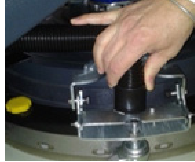
3. Check the vacuum hose is connected to the squeegee
