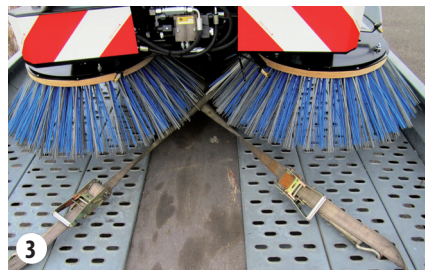
Anchoring at the front
